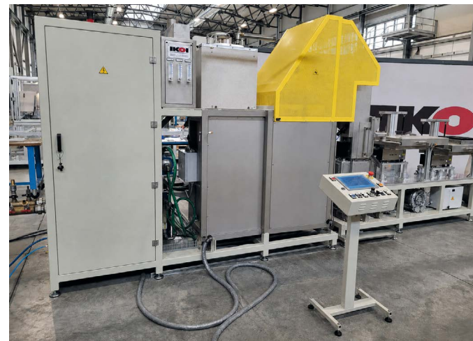
Graining machine with automatic grains extraction
