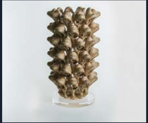
Result obtained using the lost-wax casting method
